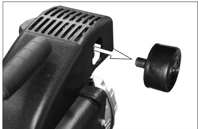
2. Remove the filter cover from the filter.
