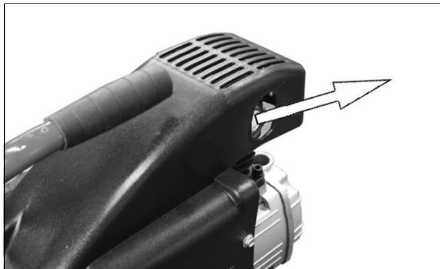
2. Screw the air filter into position.
